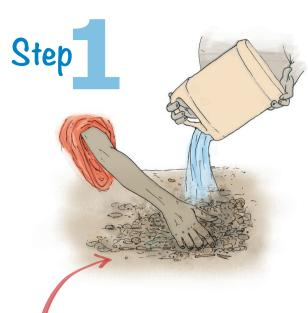
Mix animal dung with mud. Add water gradually to ensure soft mixture, stirring until the whole mixture has the same consistency. Cover the mixture and leave to sit for a day.
