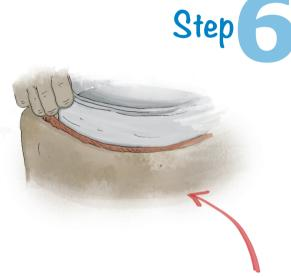
Place the cooking pot on top of the bricks. Build the wall up until just under the rim of the pot. Keep a finger-sized gap between pot and wall.
