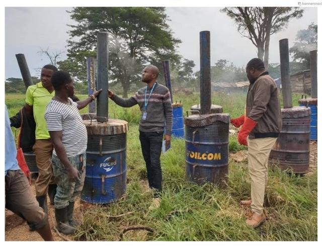
Figure 11: Metallic kilns used for char production at one of char production sites in Mvuqwe village in Kasulu District @ @UNHCR
