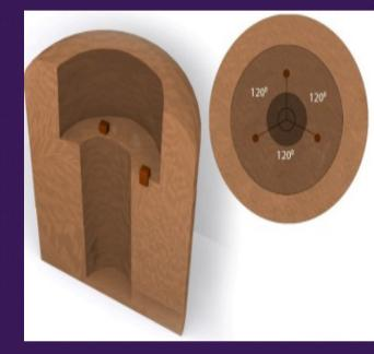
Build 3 saucepan supports inside the saucepan seat, equidistant from the centre of the combustion t to dry for 3-4 weeks and be using wet fingers to smoothen such that the stove is without cracks.
