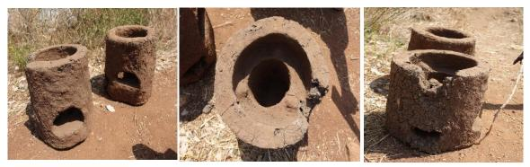
Samples of Local Mud Stoves made by ToTs Trained by GiZ showing cracking and broken saucepan cavity
