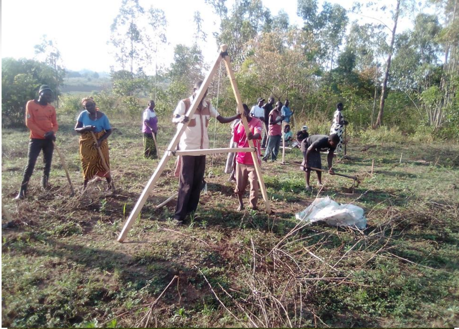
A community group using A-Frame for determining contours in a food forest site
