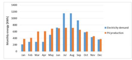
Figure 6: Energy production and consumption of a typical household with 3.6 kWp installed PV plant (Source: TTA)
