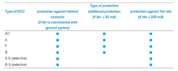
Table 7: Selection table for RCD at different type of protection (source: ABB)
