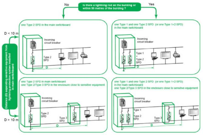
Figure 4: Quick selection guide for SPC (source: Schneider Electric)
