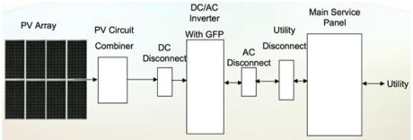
Figure 7: Minimum Equipment Required in the Installation
