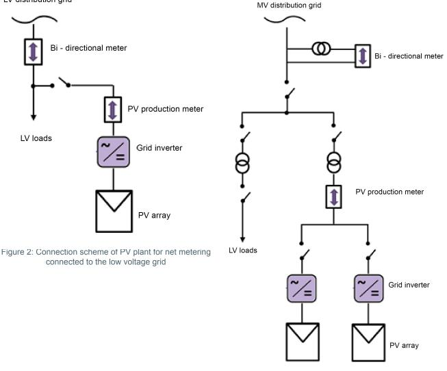
Figure 3: Connection scheme of PV plant for net metering connected to the medium voltage grid
