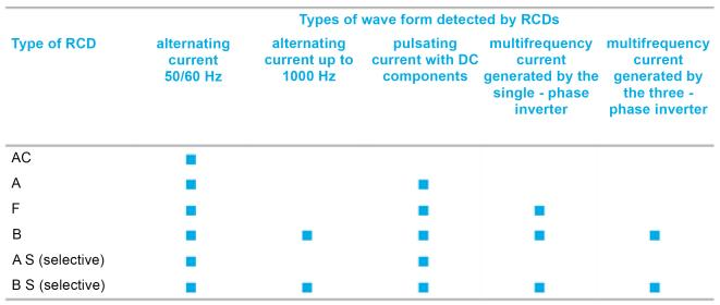
Table 8: Selection table for RCD at different waveforms (source: ABB)
