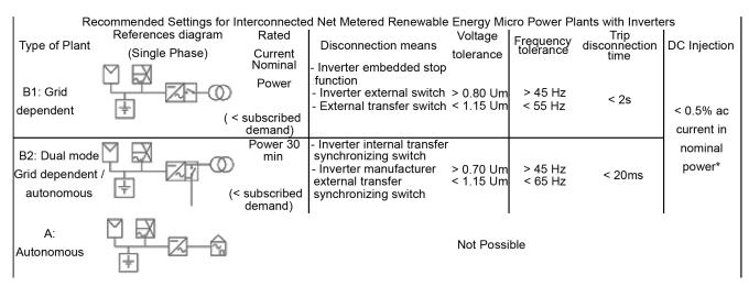
Figure 8: Recommended settings for grid-tied grid-dependent (B1), grid-tied dual mode (back-up) (B2) and autonomous plants for Lebanon (Source: CEDRO, TTA)
