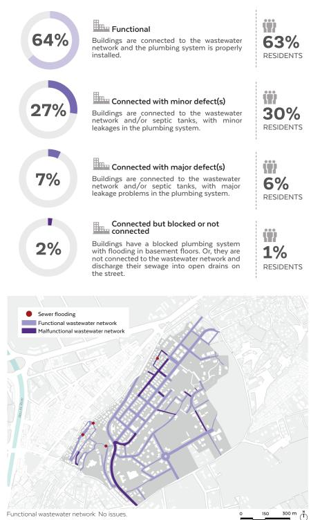
Functional wastewater network: No issues. Malfunctional wastewater network: Bad smell, flooding, recurrent clogged pipes. Figure 45 Street mapping of wastewater network
