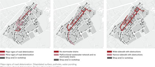
Minor signs of road deterioration: Road surface in fair condition. No stormwater drains: Lack of stormwater drains. Malfunctional wastewater network: Bad smell, flooding, recurrent clogged pipes.
