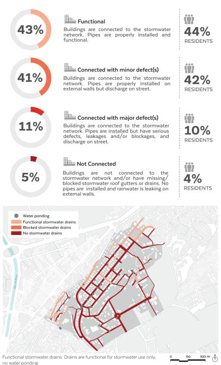
no water ponding. Blocked stormwater drains: Undersized existing drains, blocked by solid waste/mud/people's interventions/ other materials. bad smell.
