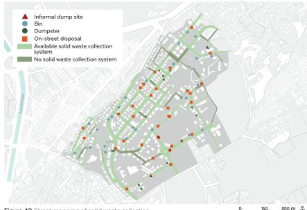
Figure 49 Street mapping of solid waste collection
